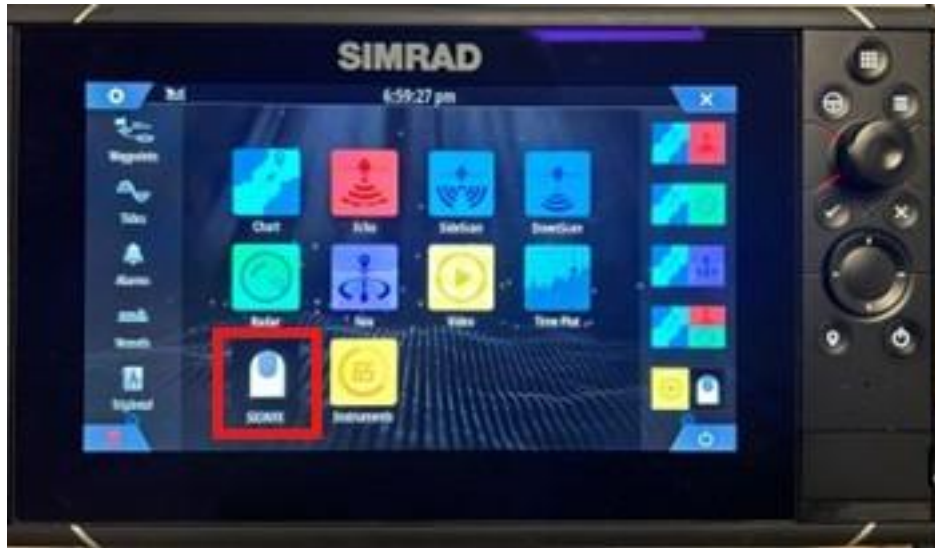
Figure 20: Accessing Camera Settings using SIMRAD MFD
