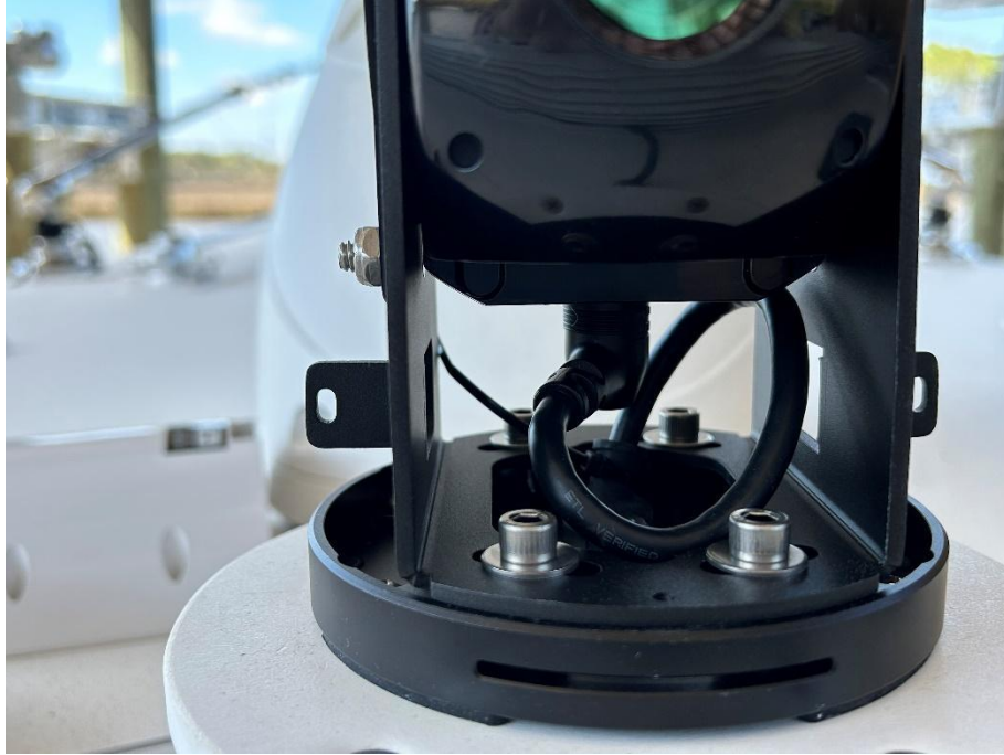
Figure 17: Camera Cable Routing Example
