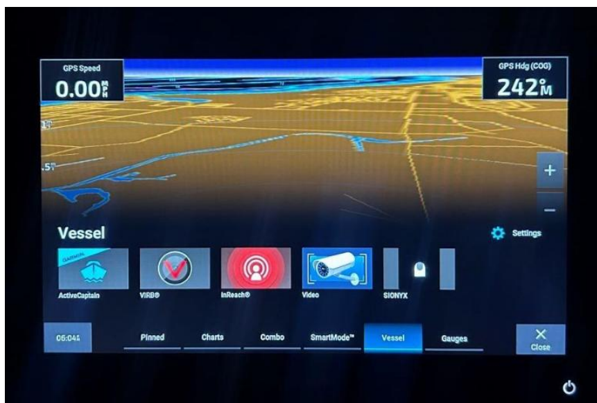
Figure 23: Accessing Video Feed Using Garmin MFD
